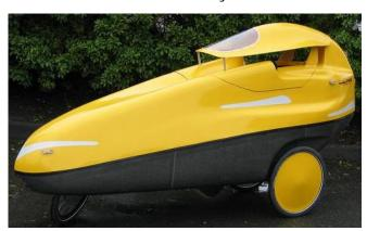
The Aurora velomobile is about 9 feet long, 32" wide, 47" high, and weighs about 79 lbs not including the electric motor and batteries. The safety equipment includes headlights (50W), a tail-light, brakelight, turn signals, a horn, dual disk brakes, as well as reflective tape all around. The yellow color also helps to ensure the vehicle is as visible as possible.
