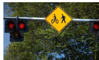
Half-signals for bicyclists should be clearly marked to minimize confusion.
