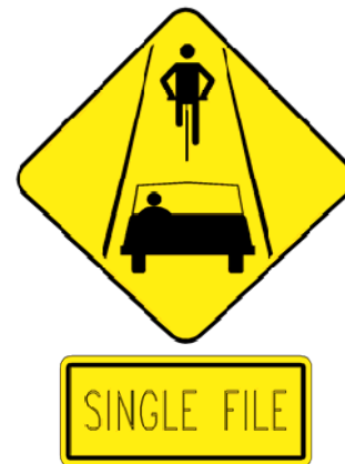
The shared use single lane single file sign is recommended in the TAC Traffic Control Guidelines (2010 DRAFT)
