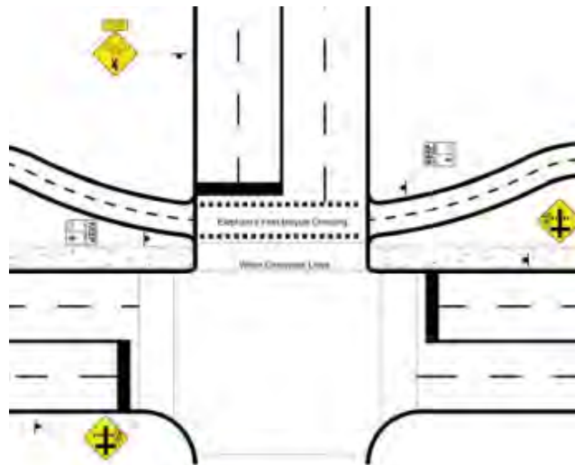
Separated at-grade crossing of a major arterial at an intersection where trail is within 75 m of a roadway intersection.
