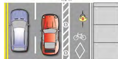
Recommended cycle track design with on-street parking.
