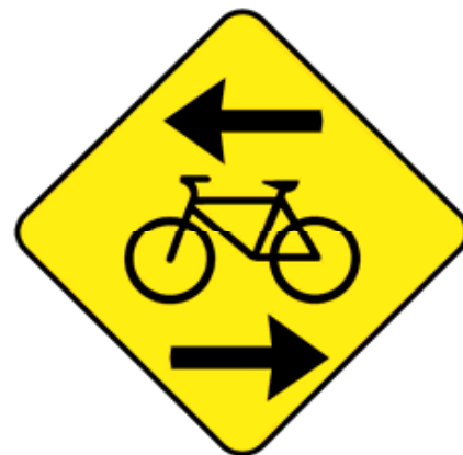
The "Contraflow Bicycle Lane Crossing Sign" (WC-XX) is recommended in the Draft 2010 TAC Bikeway Traffic Control Guidelines for use at a street crossing a bi-directional or contraflow bicycle lane.
