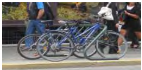
Cluster or coathanger racks can accommodate more than two bikes.
