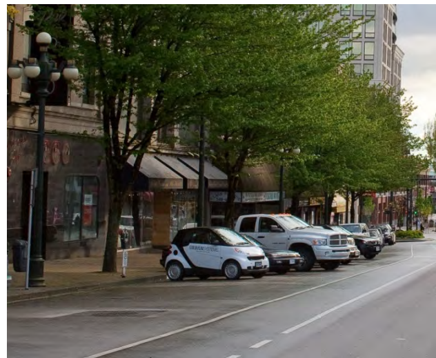
'Back-in' diagonal parking is safer for cyclists than 'head-in' diagonal parking due to drivers' visibility as they exit the parking spot (New Westminster).
