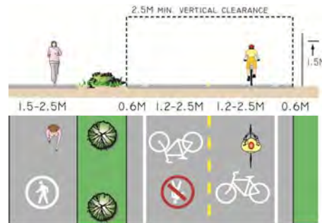
Recommended design for a separated multi-use trail.
