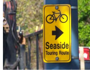
Wayfinding signage currently used in Saanich, Oak Bay and Victoria are well-liked for their visibility for cyclists, but are less visible to motorists and do not comply to TAC and MUTCD-C standards.
