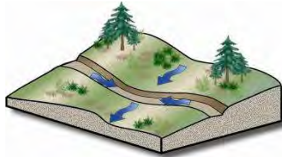
Rolling grade is the preferred design pattern for sustainable trails.
