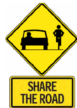
TAC signs WC-47 and WC-47S should be used in shared lanes.
