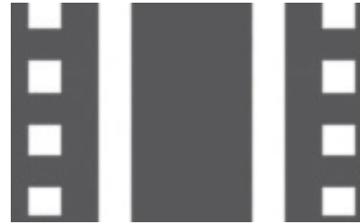
Elephants' feet indicate separated bicycle and pedestrian space at crossings.
