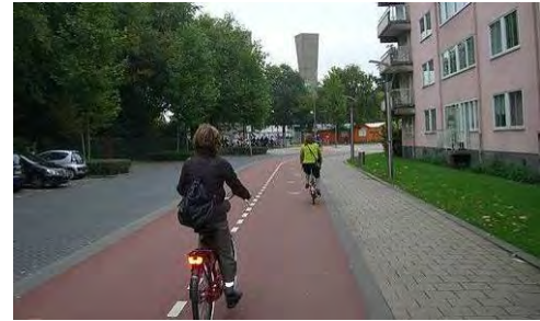
Two-way cycle track with dividing line.
